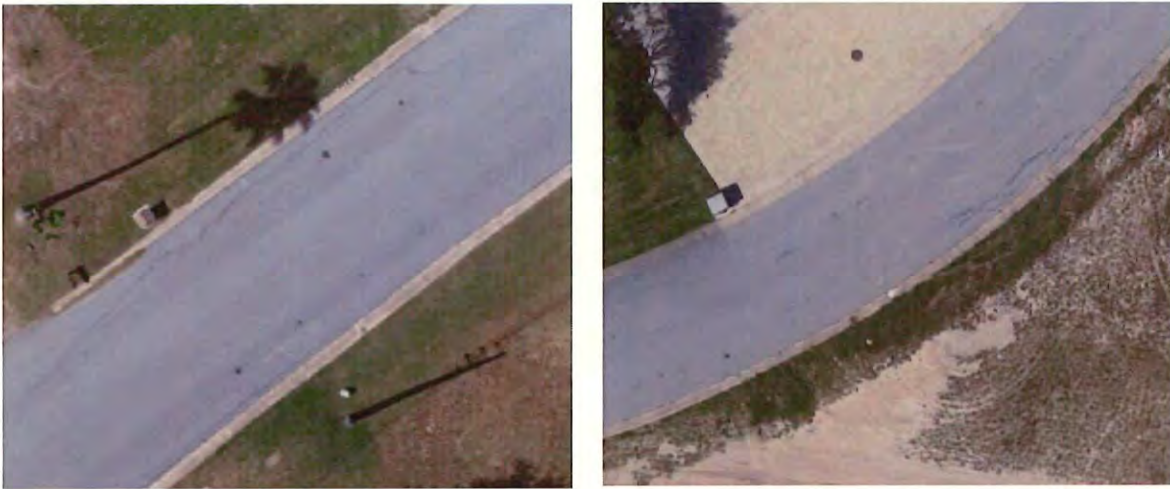
Figures 3 & 4. Examples of streets classified as being in “Good” condition. Here there is evidence of minor cracking. However, the cracking can be addressed with minor seal coating.
