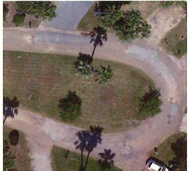
Figures 7 & 8. Examples of a street classified as being in “Poor” condition. Here there is a significant level of cracking and potholes with a higher level of separation between the cracks.
