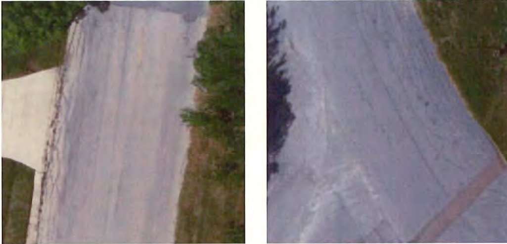
Figures 5 & 6. Examples of streets classified as being in “Fair” condition. Here there is a moderate level of cracking or deterioration throughout the whole street, however the thickness of the cracks is still relatively low.
