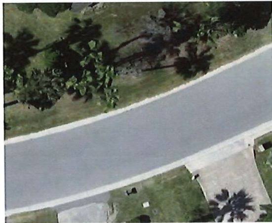
Figures 1 & 2. Examples of a street classified as being in “Very Good” condition.
